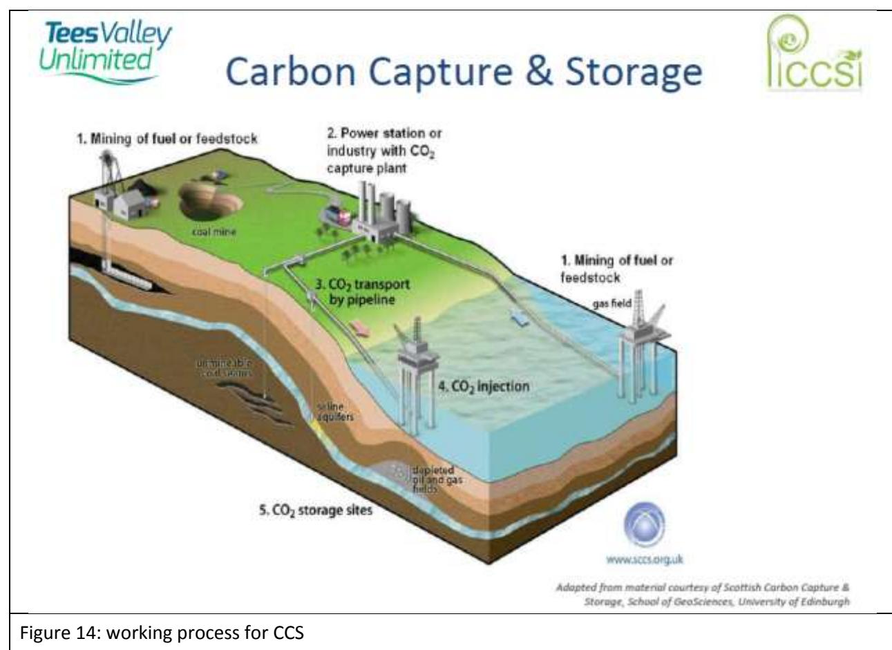
Figure 14: working process for CCS
