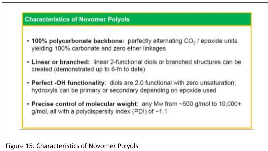
They are high performance polyols that are lower cost and more sustainable than many alternatives as shown in the figure below. Novomer products have a significantly lower carbon footprint when compared to petroleum-based polyols and other thermosets.
