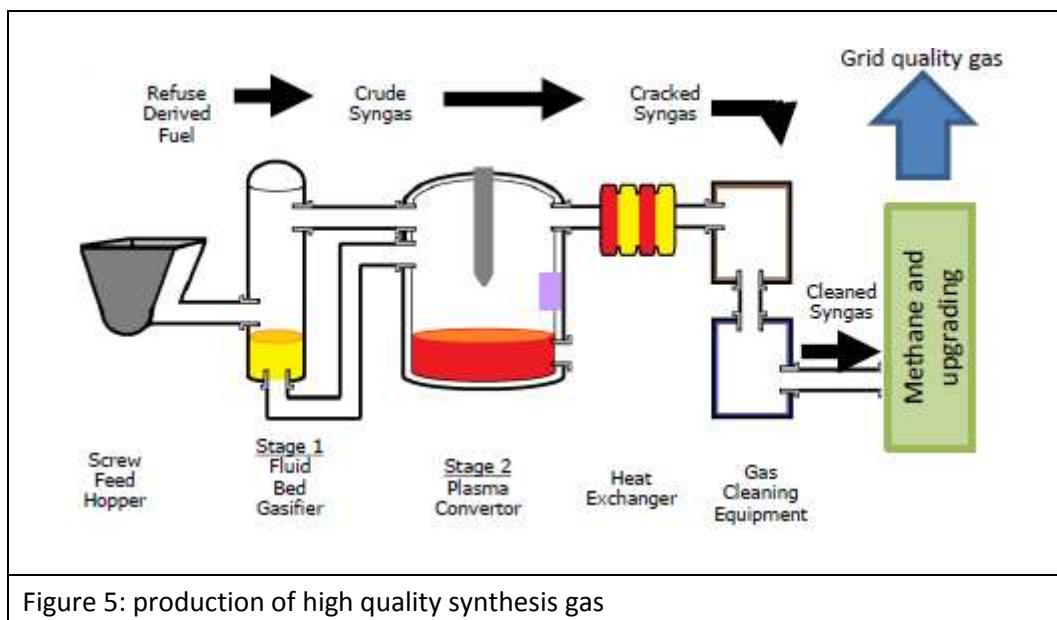
NationalGrid's involvement with a pilot project developing a commercial scale capability for the production of synthetic bio-gas was also discussed. Figure 5 above shows a system design for the provision of clean, high quality synthesis gas, Methanation at moderate scale. Confirmed projects are expected to provide heating for over 8000 homes.
